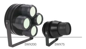
Choose from three types of filters to suit your specific application: overt illumination produces a distinct red glow that warns of the presence of IR light (715 nm), semi covert illumination produces a faint red glow that can be detected with a trained eye (850 nm) and full covert illumination avoids any red glow, making it impossible to detect the presence of IR light (950 nm)
