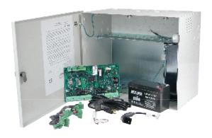
The PW-Series access modules have been designed to accommodate various mounting options. Units can be wall mounted in a high density configuration (PW5K2ENC1) when space is limited, a 19" rack configuration (PW5K2ENC2), or in a tile mount configuration (PW5K1ENC3). These controllers utilize a built-in Web server to configure the hardware attributes of the controller.
