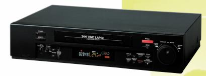
In addition to ordinary three-hour and six-hour recording modes, the KR7496E records 20 fields per second in L18H-hour mode and 4.6 fields per second in 72-hour mode, while it offers a new 96-hour mode for extending recording. To search the desired image, adjust the playback speed with the shuttle ring and search an image field-by-field with the jog dial.
