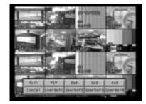
Simply move the mouse to the bottom of the main monitor screen and the various display options are shown. Choose between a full screen view, PIP (Picture in Picture), 2x2, 3x3, 4x4, or any of the four customizable userdefinable views.
