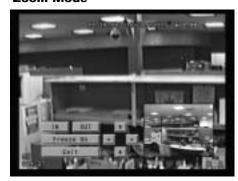
Upon selecting a camera image, a zoom screen will appear. An inset area allows you to select the portion of the image to zoom (up and down arrows), and the in/out buttons control the zoom factor. The AXMD9E provides an electronic zoom up to 32 times normal.
