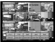
Simply move the mouse to the bottom of the main monitor screen and the various display options are shown. Choose between a full screen view, PIP (Picture in Picture), 2x2, 3x3, or any of the four customizable user-definable views.
