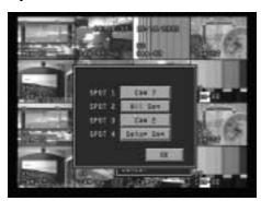
It's easy to change the contents of any of the four spot monitors. Simply select the spot monitor and select a specific camera, the entire sequence, or a user sequence.
