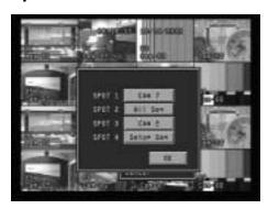
It's easy to change the contents of any of the four spot monitors. Simply select the desired spot monitor and select a specific camera, the entire sequence, or a user sequence.
