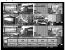
Simply move the mouse to the bottom of the main monitor screen and the various display options are shown. Choose between a full screen view, PIP (Picture in Picture), 2x2, 3x3, 4x4, or any of the four customizable user-definable views.
