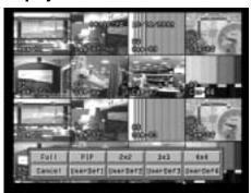
Simply move the mouse to the bottom of the main monitor screen and the various display options are shown. Choose between a full screen view, PIP1, PIP2, PIP3 (Picture in Picture), 2x2 or any of the four customizable user-definable views.
