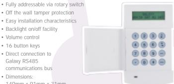
All Galaxy peripherals are connected directly to the Galaxy RS485 communications bus. All accessories are fully compatible with the full range of Galaxy control panels. The Galaxy 16 and 16 plus range is fully compatible and interchangeable with the Galaxy 8, 18, 60, 128, 500, 504 and 512 control panels.
