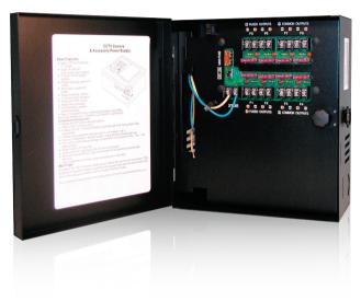
The PWR-24AC-8-4UL is a UL listed CCTV power center engineered to manage remote camera and accessory power requirements. The PWR-24AC-8-4UL distribution module is designed with 8 individually fused outputs for powering up to 8 CCTV cameras and accessories. It will provide 24Volts AC via distribution to eight fused outputs with a total of 4.0 Amps continuous supply current. The PWR-24AC-8-4UL power center is housed in a premium heavy gauge metal enclosure.
