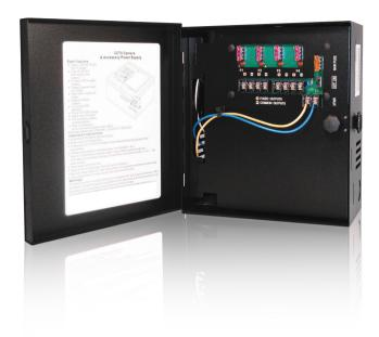
The PWR-12DC-4-5 is a CCTV power center engineered to manage remote camera and accessory power requirements. The PWR-12DC-4-5 distribution module is designed with 4 individually fused outputs for powering up to 4 CCTV cameras and accessories. It will provide 12 VDC via distribution to four fused outputs with a total of 5 Amps continuous supply current. The PWR-12DC-4-5 power center is housed in a premium lockable heavy gauge metal enclosure.
