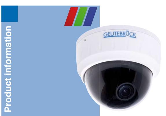
High resolution WDR-PIXIM 1/3" color fix dome in housing made of molded plastic with integrated lens and adjustable focal length from 3.0 - 9.0 mm. The camera is equipped with automatic white balancing (AWB) and provides an on screen setup function. Because of itis flexible 3 axial camera modul adjustment the dome can be fixed to any normal or angular ceiling and even directly on the wall.
