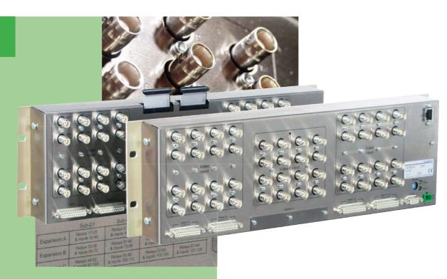
Networkable, freely programmable video matrix including powerful management software for use in combination with an external control PC. Basic matrix unit with 32 video in- and 16 outputs and 32 contact in- and 16 relay outputs, controlled via serial or LAN interface by any PC. Extendable by one, CX3 Extension 32' up to 64 video in- and 16 outputs as well as 64 contact in- and 32 relay outputs.
