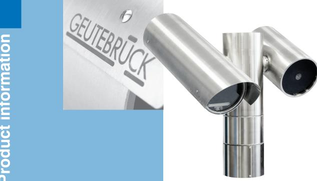
High performance infrared illuminator for the high precision pan-tiltcamera unit ARGUS. The stainless steel housing of the infrared illuminator will be mounted in opposite to the camera housing on the tilt axis of the pan-tilt-unit and is equipped with an easy connection flange for a simple and quick installation process. With the illuminators high performance infrared LED's the ARGUS-system can perform at itïs best both under daylight and under night-time condi-
