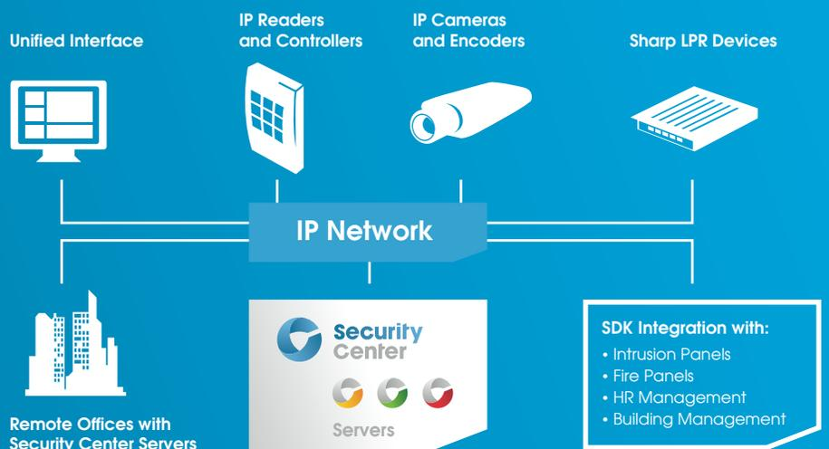
**Solution Components.** The Security Center merges three main security applications including license plate recognition, video surveillance and access control in one innovative solution. But innovation doesn't stop there.
