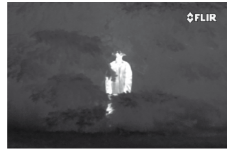
Thermal imaging: suspect hiding in bushes is clearly visible since thermal contrast is practically impossible to mask.
