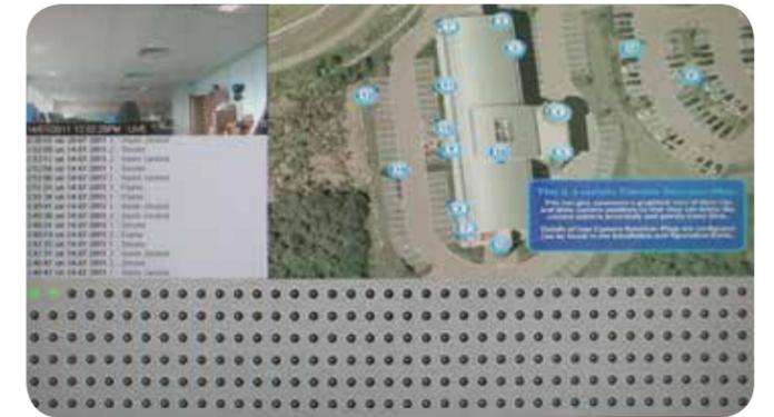
Alarm verification, acceptance and clearance is provided through either a mouse connected to the FireVu Annunciator or the use of touch screen technology. The user is also able to view live video from any camera on the site map by simply selecting that camera's LED or location label from the site map.
