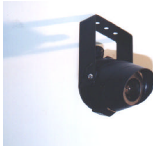
Above: A black EX10 with a clear (non-tinted) window can be installed to black ceilings in commercial and industrial locations for discrete surveillance without loss of any lux levels.
