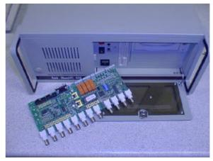
Alarm Trigger - The EIV will interface via relay switches with other Building Management systems such as fire, security or environmental control. A series of 'pre-trigger' frames may also be stored. Trigger can also be assigned as a 'raid' event causing the video frames to be recorded as true bitmap images at up to 10 frames per second.
