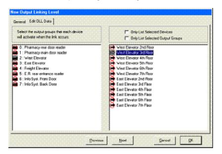
Each Output in the Linking Group has a Time Zone that determines what times and days the output will activate when linked to. This provides a means to give different cardholders or even the same card holder different windows of access, (defined by time and day), for each Floor Select Button.
