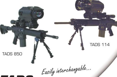
The TADS systems offers night vision in complete darkness through the weapon's day-sight using uncooled 8-12µm microbolometer focal plane array technology. DiOP utilizes its proprietary signal processing techniques, which produce thermal images of unsurpassed quality for an uncooled thermal imaging product.
