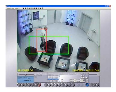
The SmartFinder, a system for the intelligent search for objects within a picture, allows for a fast and efficient evaluation of the recorded data in any area of the picture.
