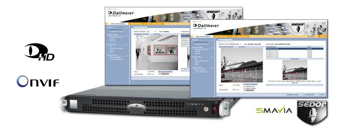
The DVS 2200 IPS is a high-performance SEDOR® video analysis server appliance for the analysis of up to 12 IP video channels and the recording of up to 24 IP video channels.
