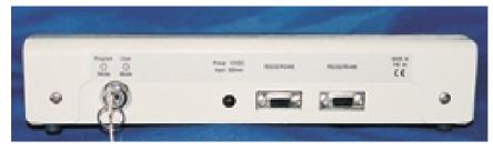
Rear panel of keyboard showing program switch, power jack and 2 RS485 / RS232 Ports. Power input 12V dc, 300 mA
