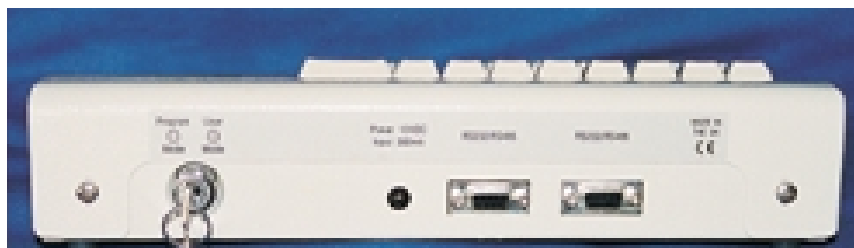
Rear panel of keyboard showing program switch, power jack and 2 RS485 / RS232 Ports. Power input 12V dc, 300 mA
