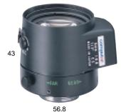
HG0808FCS-HSP HG0808AFCS-HSP Product Code DD Iris Focal Length 8mm 8mm F0.8-360 F Stop F0.8-360 44.9° Angle (h) 44.9° Plugged Type 120g Weight 130g -10 - +50°C -10 - +50°C Operating Temp. Filter Size 40.5mm 40.5mm
