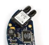
The ComNet™ series of Ethernet media converters are designed to transmit and receive 10/100 Mbps data over one or two multimode or single mode optical fibers. They are designed to be mounted within an Aigis dome and provide optical Ethernet connectivity.
