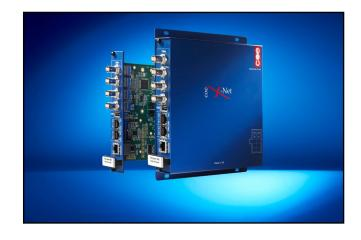
Utilising the latest H.264 Main Profile compression algorithm, X-Stream 400 delivers superior picture quality at reduced bandwidth across any Ethernet network. By providing digital compression and encoding for up to 4 channels of analogue video, as well as data, audio & contact closure interfaces, X-Stream 400 is a fully featured and highly cost-effective video transmission solution.
