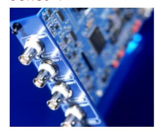
The COE Series 4 is a digital 4 channel video multiplexer, with optional duplex auxiliary channel, for use with optical fibre networks
