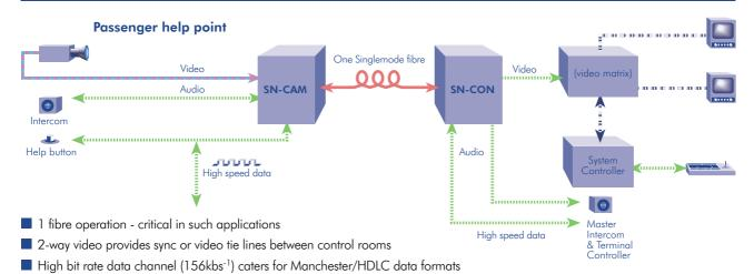
**Transport systems:** The high path loss capabilities offer transmission up to 40km for metro, road and rail applications. High performance video maximises the camera-monitor signal link quality. The data and stereo audio channels allow the COE S-class to be used in passenger help points providing an integrated, single fibre solution.
