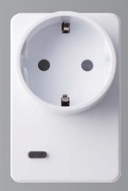
The PSMD-29ZBS ZigBee power meter plus dimmer switch series is designed for the user to remotely dim or turn on/off incandescent light via a smartphone or web browser anytime, anywhere. The PSMD-29ZBS series has a built-in power meter to measure electricity consumption, allowing users to review their usage history over the day / week / month for energy saving purposes.
