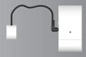
EMD-1ZW is a smart power metering device designed to measure electricity consumption from the electricity meter. E-Meter counts LED pulses from the house meter and converts it to Watt and accumulated KWh. Measuring your home's energy consumption is the first and most important step toward reducing energy consumption and achieving greater energy efficiency.
