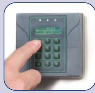
The InfoProx reader controls local door strikes or other equipment without the need for a separate door controller.
