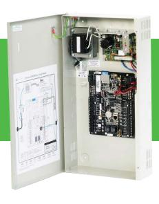
The sDCM 300 (Door Control Module) is a low cost, two-door controller designed to interface third-party read heads with the CEM range of access control systems.
