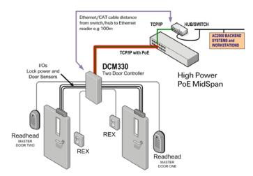
The PoE+ injector or mid span device supplies all the power for the devices and locks required by two doors.
