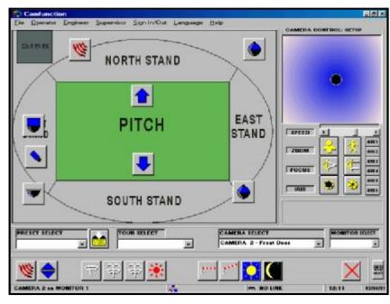
CAMFUNCTION also offers VCR/Digital recorder controls, allowing integration of the whole CCTV system through a single on-screen interface. This reduces the desk top space required and allows the VCR to be positioned in a secure area.
