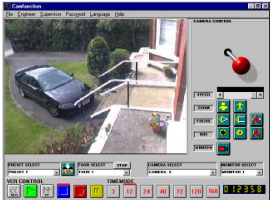
CAMFUNCTION also offers VCR controls, allowing integration of the whole CCTV system through a single on-screen interface. This reduces the desk top space required and allows the VCR to be positioned in a secure area.
