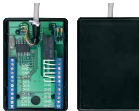
ALARM81-RS: external RS-232 alarm box with 8 alarm inputs and 1 relays output
