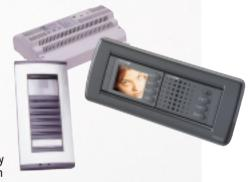
207x99x28mm together with the most highly specified colour monitor on the market with its recessed back box measuring just 174.3wx59hx49.8mm, it has a 2" screen, a lock release, monitor live and 2 aux buttons, brightness and colour controls plus an audio button. The kit is complete with a VA/200 combined control unit and PSU.
