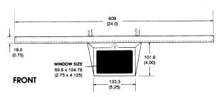
Dimensions in millimeters. Dimensions in parentheses are in inches.
