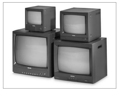
Designed for ease of installation and operation, the monitors will accept a voltage supply of 100-230 VAC, without the need for any switching or adjustments. The monitors are setup for standard composite video signals, the LTC -/5x versions CCIR format, the LTC -/6x versions EIA format and the LTC 2020/90 with automatic detection of CCIR/EIA format.
