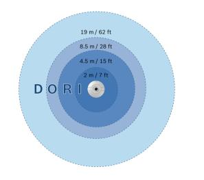
When mounted at a height of 3 m (10 ft) the  $180^{\circ}$  version of the camera has the following coverage radius for the four levels:
