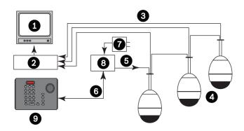
Typical Multiple Camera Sites using Daisy Chain Bi-Phase Control Code Wiring Configuration
