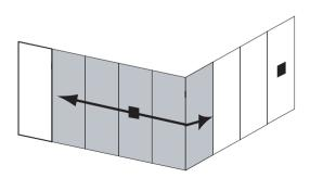
Weld wall/wall corner connection end to end
