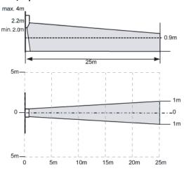
The detector requires a stable reference for the entire detection zone. The detection zone consists of two subzones (separated by the central level). The subzones cannot be referenced to different surfaces that may consist of differing materials. The middle level of a detection zone is in the detector's longitudinal axis, which is perpendicular to the installation surface (housing floor).
