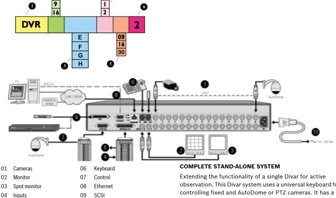
observation. This Divar system uses a universal keyboard for controlling fixed and AutoDome or PTZ cameras. It has a main monitor plus spot monitor, alarm I/O (for external alarms and sensors), a storage array and a PC with Control Center software. A DVD writer is used for making archives. An ATM/POS bridge can be used to connect to an ATM or point-of-sale machine.
