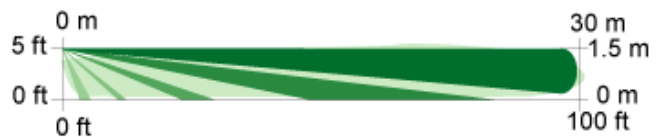
Side View Optional Long Range Coverage (DS970): 30 m x 3 m (100 ft x 10 ft)
