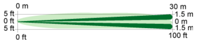
Top View Optional Long Range Coverage (DS970): 30 m x 3 m (100 ft x 10 ft)
