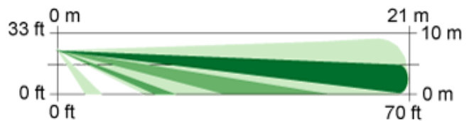
Side View Standard Broad Coverage (DS970): 21 m x 21 m (70 ft x 70 ft)
