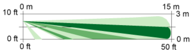
Side View Standard Broad Coverage (DS950): 15 m x 15 m (50 ft x 50 ft)
