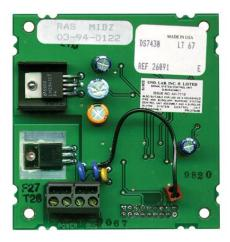
The DS7430 is a Multiplex Expansion Module for use with the DS7400Xi Series control panels. It connects directly to the control panel and provides a two-wire multiplex bus for the connection of up to 120 multiplex sensors and interface modules.
