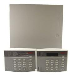
The DS7240V2 Control Panel has eight zones expandable to 40, four outputs expandable to 20, and four areas. It is suitable for commercial burglary and residential fire/burglary applications.
