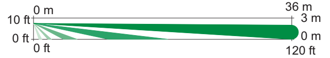
Side View Optional Long Range Coverage: (OMLR77) 40 m x 3 m (120 ft x 10 ft)
