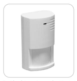
The DS940Q is a wall mount, Quad Passive Infrared Intrusion Detector. This detector employs two individual sensors which operate like two PIRs in one. Each sensor is processed separately and both must activate to cause an alarm.
